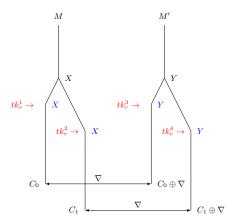
Fig. 20: RTK boomerang attack against forkcipher producing forgery for single block. Here  $tk_r^1$  and  $tk_r^2$  are two round keys after forking which introduce the tweakey difference. X and Y are states of the ForkSkinny after forking.
