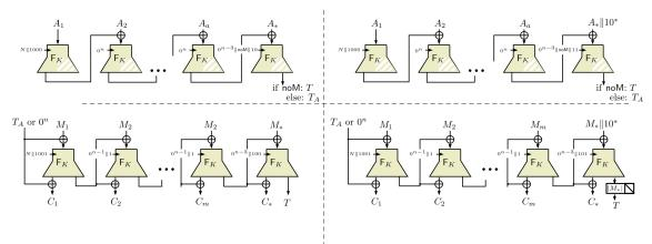
Fig. 7: The encryption algorithm of SAEF[F] mode. The bit noM = 1 iff |M| = 0. The picture illustrates the processing of AD when length of AD is a multiple of n (top left) and when the length of AD is not a multiple of n (top right), and the processing of the message when length of the message is a multiple of n (bottom left) and when the length of message is not a multiple of n (bottom right). The white hatching denotes that an output block is not computed.
