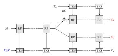
Fig. 3: ForkSkinny encryption with selector s = b. A plaintext M, a key K and a tweak T (blue) are used to compute a ciphertext  $C = C_0 || C_1$  (red) of twice the size of the plaintext. RF is a single round function of SKINNY and TKS is round tweakey update function [17], and BC is a branch constant that we introduce.
