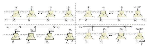
Fig. 9: The encryption algorithm of RPAEF[F] mode. The picture illustrates the processing of AD when length of AD is a multiple of n (top left) and when the length of AD is not a multiple of n (top right), and the processing of the message when length of the message is a multiple of n (bottom left) and when the length of message is not a multiple of n (bottom right). The white hatching denotes that an output block is not computed.
